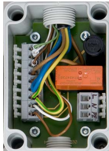
Connection Box Pump
